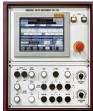
■ CNC Control Panel
